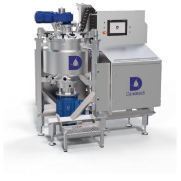
and into the mixer below liquid level, and it is instantly wetted. The powerful high-shear mixer and scraper agitator generates a controlled vortex in the tank. The combination of vortex and vacuum effectively separates air from liquid and generates a perfect homogenous dispersion within seconds. The unit comes with an isolated jacket for fast heating and cooling with steam or ice water. For extra quick heating, the unit is equipped with a direct steam valve.
