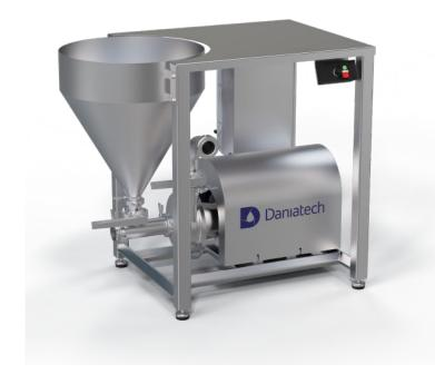
During operation, the mixing wheel accelerates the liquid and creates pressure through in the injector pipe, which sucks in powder from the powder funnel. The amount of powder is controlled by a manual butterfly valve.
