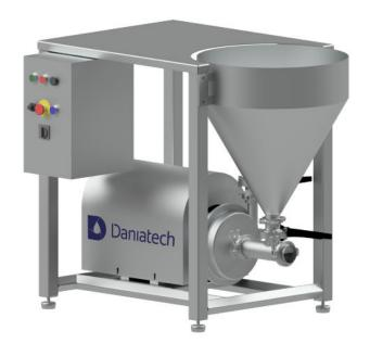
During operation, the mixing wheel accelerates the liquid and creates pressure through in the injector pipe, which sucks in powder from the powder funnel. The amount of powder is controlled by a manual butterfly valve.
